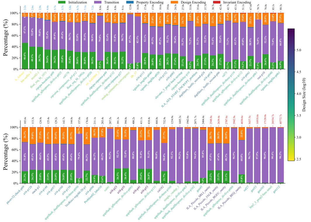
Fig. 5. The percentage breakdown of Initialization, Transition, Property & Invariant Encoding, and Design Encoding times for each design instance. End-to-end execution times are shown above each bar, sorted in ascending order. X-axis labels are colored according to the logarithm of design size using the colormap shown at right, where darker colors correspond to larger designs.
